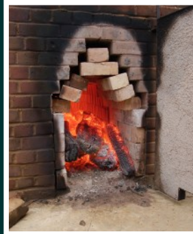
Wood fired kiln
