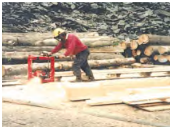
Plate 4. Chainsaw mill in action Forestry Commission
