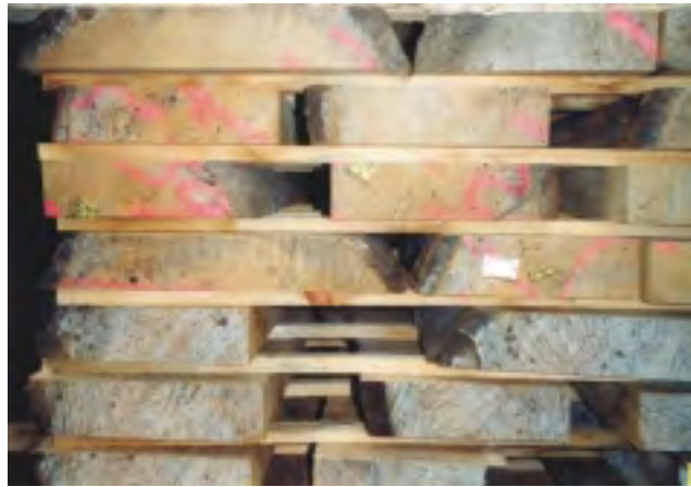
Plate 9: Leave spaces between boards in each layer
