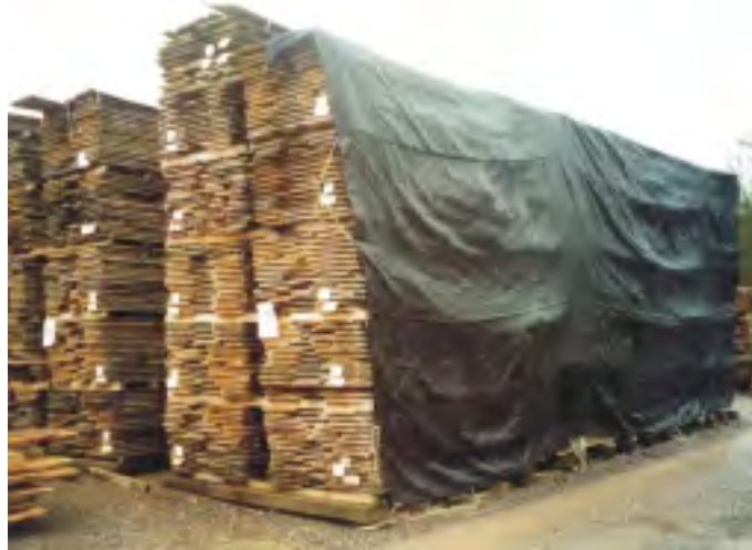
Plate 11: Shade cloths protecting lifts of drying timber
