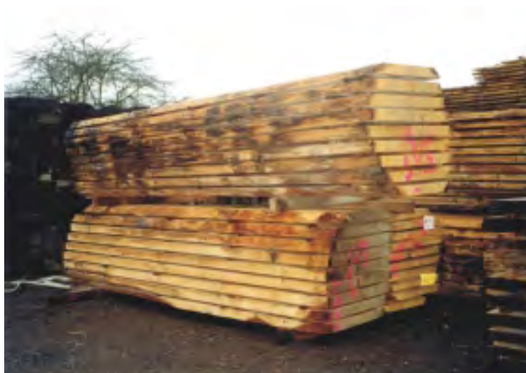
Plate 12: Piling in log form
