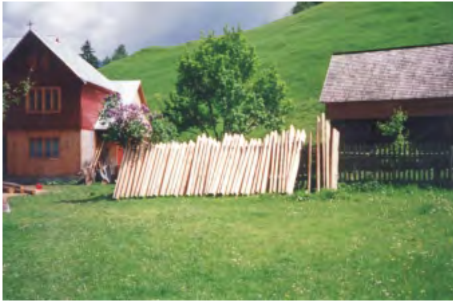
Plate 13: End racking timber using a fence
