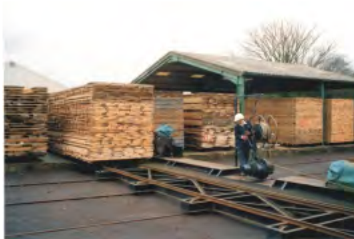
Plate 4: A charge of timber for kilning, Timbmet Ltd, Oxford
