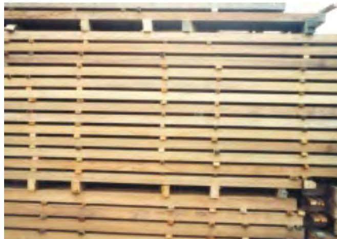
Plate 7: Align stickers with supporting timbers and use appropriate spacing
