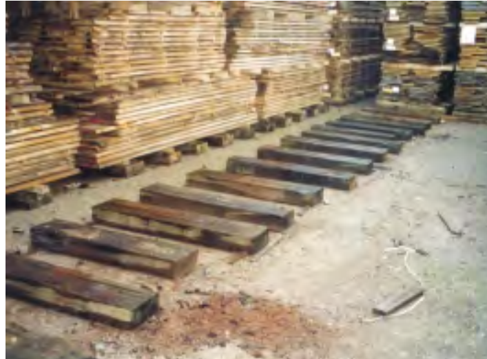
Plate 6: A well packed hardcore base with timber sleepers
