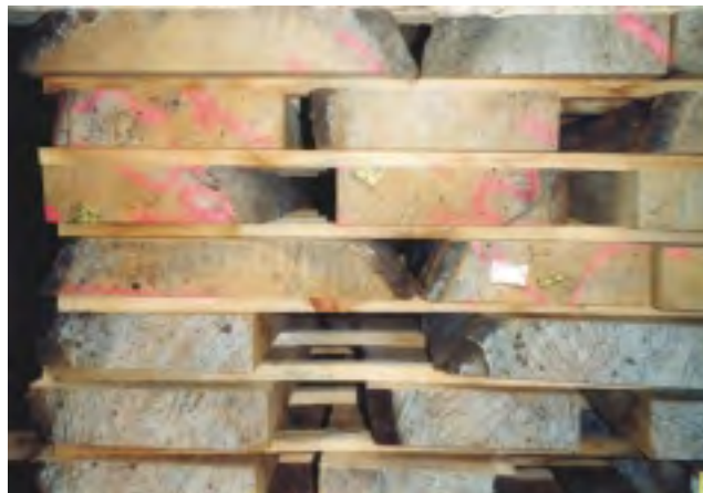
Plate 9: Leave spaces between boards in each layer
