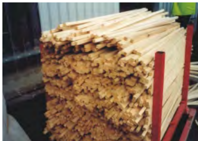
Plate 8: Dry softwood stickers used for separating each layer of timber
