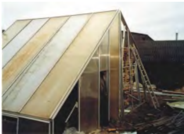
Plate 5: A solar drying unit being filled with timber
